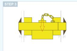
Push Pin into Lock shaft
